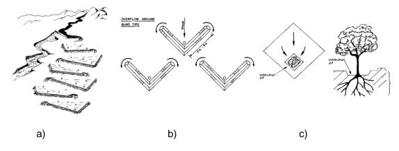
Figure 10: Examples of Water harvesting a) Flow diversion system b) V-shaped and c) Negarim microcatchment (edited, accoarding to Critchley and Siegert, 1991)
