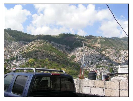
Issue: Land clearing, deforestation and surface sealing for building on slopes in PAP Recommendation: Infiltrating the rainwater where it falls, so that it doesn't accumulate and floods downstream, Retention in ponds for irrigation on higher elevations, terracing and reforestation, ravine restoration,
